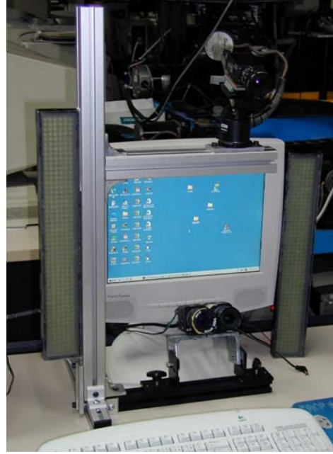
Fig. 4: The stereo eye tracking system.
