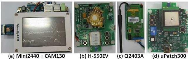
Figure 3: VS<sup>3</sup> hardware components.
