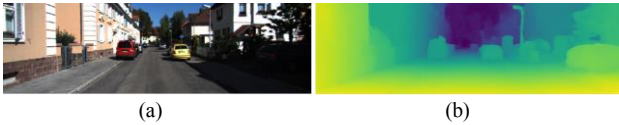
Fig. 1. An example of the pre-processed depth maps on KITTI dataset. (a) Input image. (b) Depth map generated by PSMNet.
