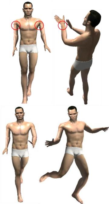
Figure 7. Skinning artifacts. Upper: with lower voxelization resolution (1072 particles): lower: with higher voxelization
