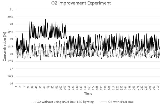
Fig. 6. Experiment of O<sub>2</sub> improvement inside the IPCH-Box.
