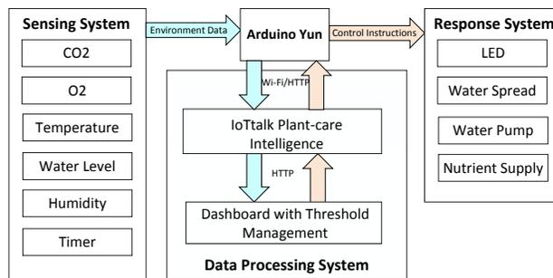
Fig. 3. The functional block diagram of IPCH-Box.
