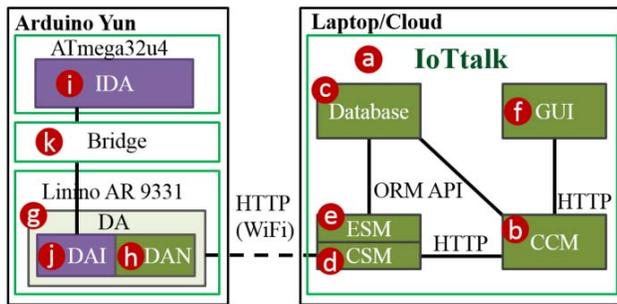
Fig. 1. The IoTtalk architecture.
