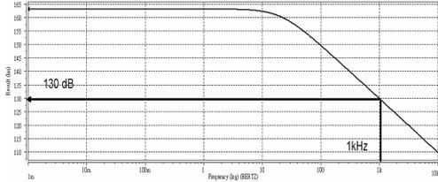
Figure 8. CMRR performance of the current-balancing IA.
