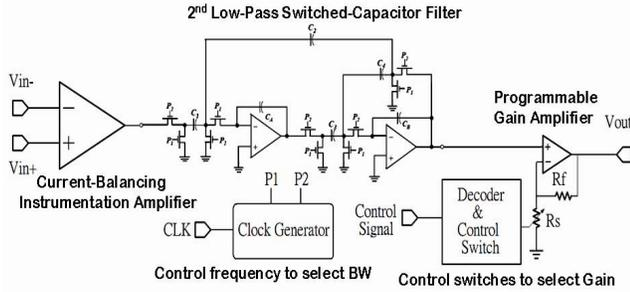
Figure 2. Architecture of the analog front-end circuit design.
