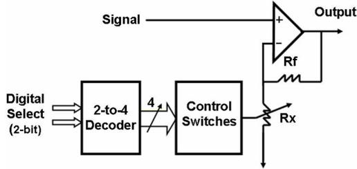
Figure 5. Architecture of the programmable gain filter.
