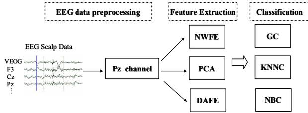
Figure 2. System flowchart for processing the ERP signals.
