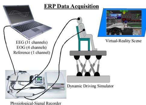
Figure 1. Physiological signal measurement system with kinesthetic/visual/auditory stimuli in the 3D dynamic VR-based traffic-light motion simulation experiments.
