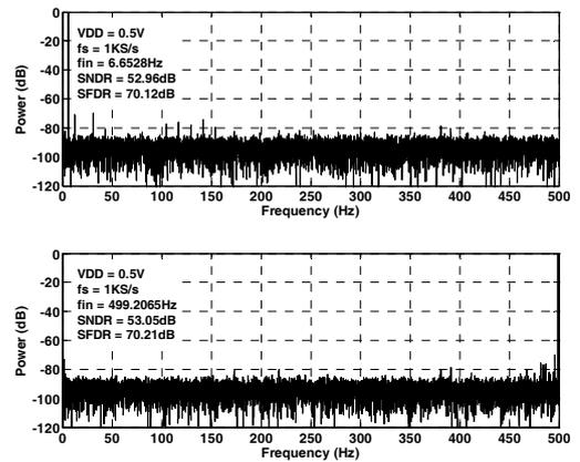
Fig. 6. Measured output spectrums at 1KS/s with a 0.5V supply.
