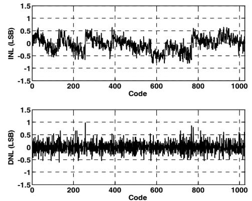
Fig. 5. Measured INL and DNL at 1KS/s with a 0.5V supply.
