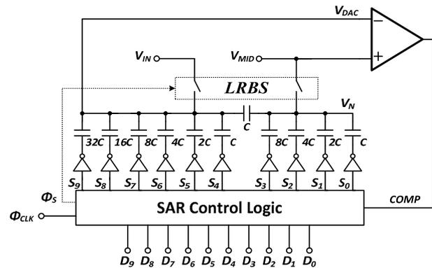
Fig. 1. SAR ADC architecture with the proposed LRBS.
