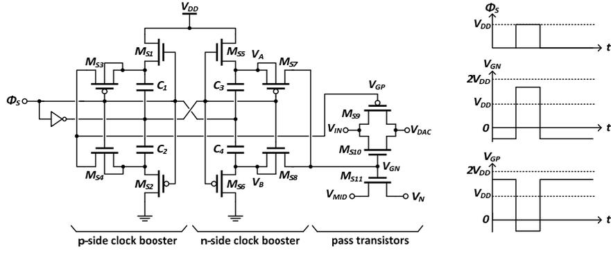
Fig. 2. Proposed LRBS schematic and waveforms of the original and boosted clock.
